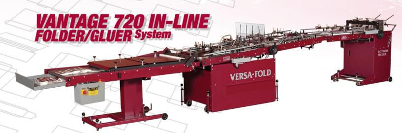
The Vantage 720 System is an in-line Folder/Gluer with an impressive production rate (speeds up to 22,000 cartons per hour). The Vantage 720 System is ideally suited for producing straight-line boxes, room key holders, table tents, sleeves, CD wallets, computer software cartons and presentation folders. An optional kit for producing auto-lock bottom boxes is available.
