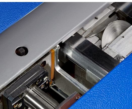
EVA/Hotmelt Side Gluing
